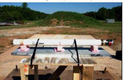
FIGURE 6. Fragment Impact Test Setup
