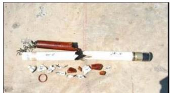
FIGURE 8. Composite Case Debris
